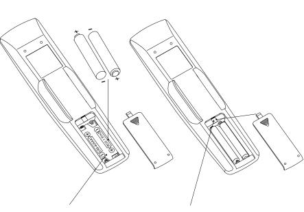
Press in and lift tab to remove battery cover out of recess.
